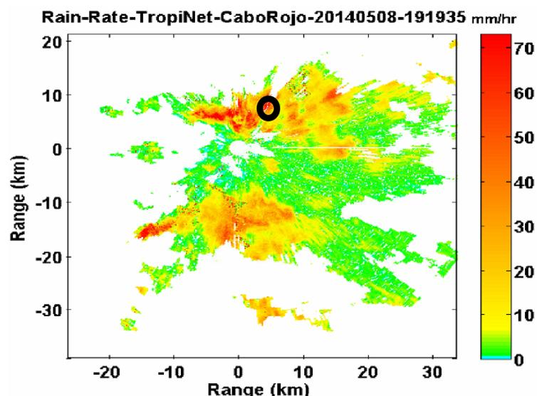
Figure 1: Rainfall Rate for TropiNet Cabo Rojo with polarimetric variables  $K_{DP}$  and  $Z_{DR}$ , and circle shows the UPRM disdrometer.
