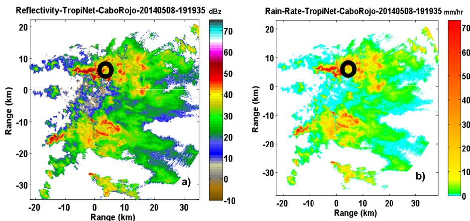
Figure 1: TropiNet Cabo Rojo Data: a) Reflectivity and b) Rainfall Rate; circle shows the disdrometer location
