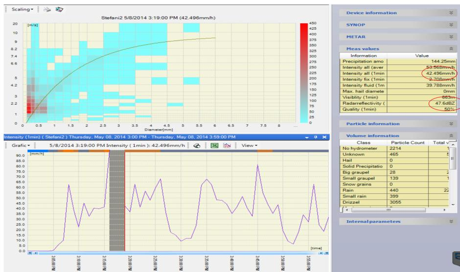
Figure 2: Thies Clima Disdrometer Display; circles shows the radar reflectivity and the precipitation intensity
